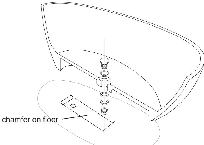
3. Align the expansion joint and glue the silicone tightly with the drainage
