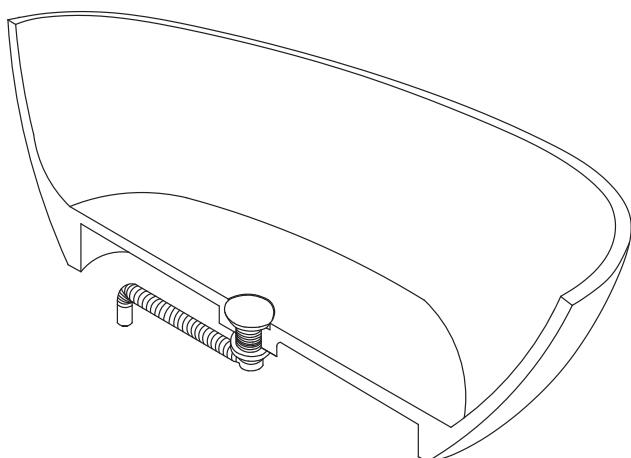
5. Fixing the bathtub on the floor with glass cement to make sure it's sealed. Half hour later, fill in water to the bathtub and drain out from the bottom to make sure all joints are watertight.
