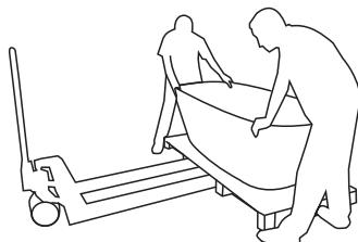
3. Carefully move the bathtub from the wooden pallet to the forklift manually.
